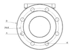
D = Flange diameter Hcd = Hole circle diameter d = Diameter of bolt holes n = Number of bolt holes
