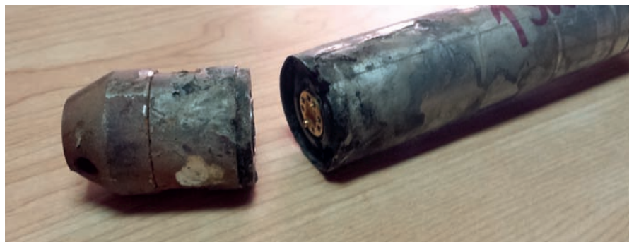
Sensor body: Electro-chemical corrosion (ballast tank)
