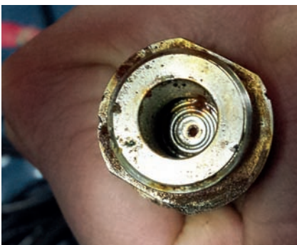
Sensor membrane: Mechanical damage
